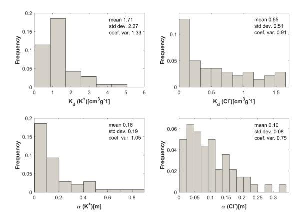
Fig. 3.14 Histograms and basic statistics of dispersivity and partition coefficient for Cl<sup>-</sup> and K<sup>+</sup>
