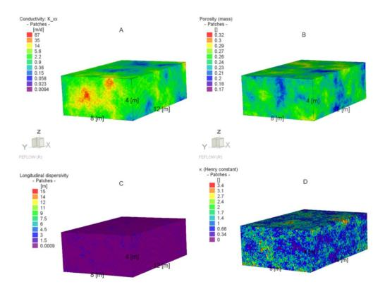
Fig. 5.2 Realizations number 1 of ln K (A), n (B), ln  $\alpha$  (C) and k (D) at fine scale
