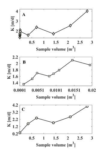
Fig. 3.13 Variation of K with measurement scale A) all tests; B) only laboratory tests; C) only field tests (DRI and ditch infiltration)
