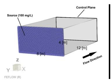
Fig. 5.3 Sketch of solute transport models indicating the source zone (purple rectangle) and the exit control plane where mass concentration was measured.
