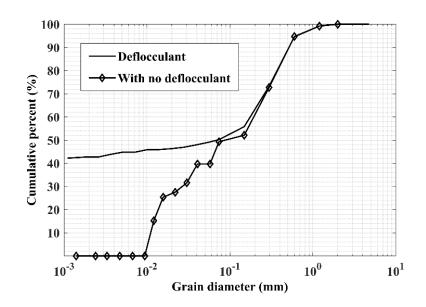
Fig. 3.7 Granulometric curves for soil samples prepared with and without deflocculant
