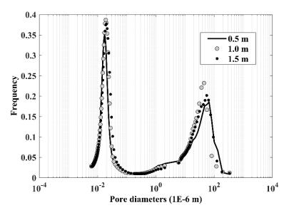
Fig. 3.6 Results of three MIP tests: frequency of pore diameters for samples taken at 0.5 m, 1.0 m and 1.5 m depth
