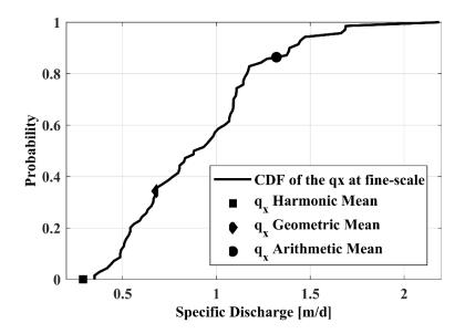
Fig. 4.8 Cumulative frequency distribution function of  $q_x$  at the fine-scale and  $q_x$  values obtained for a homogeneous formation with conductivity equal to the harmonic, geometric and arithmetic means
