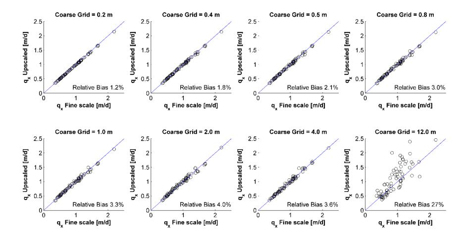
Fig. 4.5 Comparison of the specific discharge in the x-direction  $(q_x)$  through a plane orthogonal to the flow direction obtained from the model at the fine scale *versus* the results obtained from the models at coarser scales after computing the block values using the Laplacian-with-skin method
