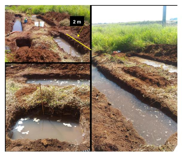
Fig. 3.5 Infiltration in rectangular ditches in progress
