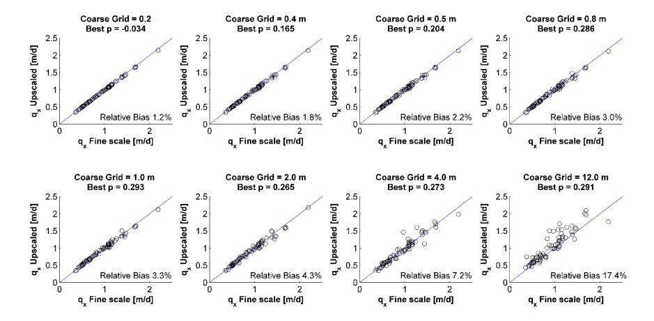
Fig. 4.10 Comparison of the specific discharge in the x-direction (q<sub>x</sub>) obtained from the model performed at the fine-scale *versus* the results obtained from the models at coarser scales after computing the block values using p-norm average with the best p - exponent
