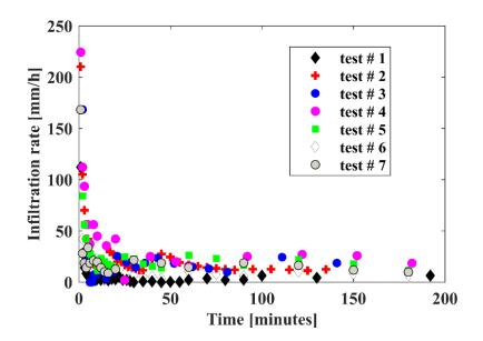
Fig. 3.10 Results of seven double-ring infiltrometer tests
