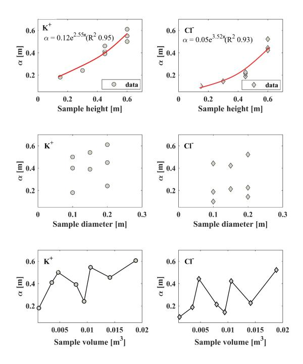
Fig. 3.18 Variation of the dispersivity of K<sup>+</sup> and Cl<sup>-</sup> with sample height, diameter and volume
