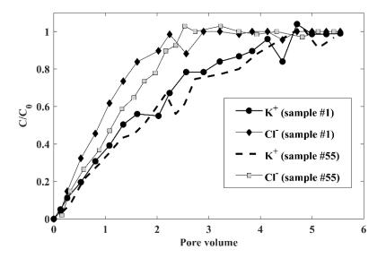
Fig. 3.15 Breakthrough curves of Cl<sup>-</sup> and K<sup>+</sup> for two miscible displacement experiments performed in small-scale samples
