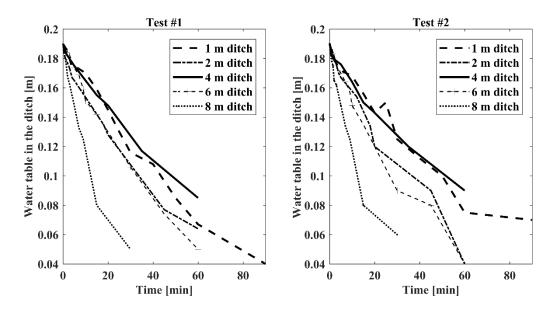
Fig. 3.12 Evolution of the water table in the ditches with time in test 1 and 2
