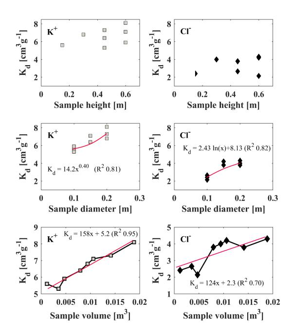
Fig. 3.19 Variation of the partition coefficient of K<sup>+</sup> and Cl<sup>-</sup> with sample height, diameter and volume
