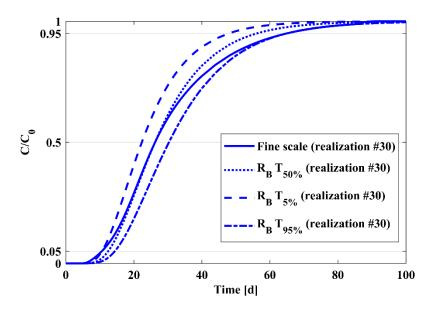
Fig. 5.14 Breakthrough curves for realization number 30 at the fine and coarse scales using the best p exponent for this specific realization, and considering three different retardation factors depending on whether the focus is in predicting the early, median or late arrival times
