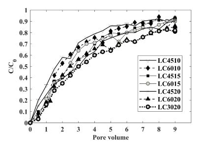
Fig. 3.16 Breakthrough curves of K<sup>+</sup> from one of the miscible displacement experiments in each large-scale sample size
