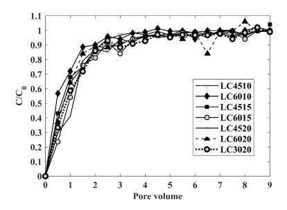
Fig. 3.17 Breakthrough curves of Cl<sup>-</sup> from one of the miscible displacement experiments in each large-scale sample size
