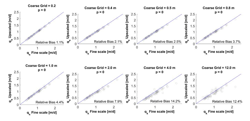
Fig. 4.13 Relative bias of the  $q_x$  obtained with blocks computed using p-norm with p = 0 (geometric mean)
