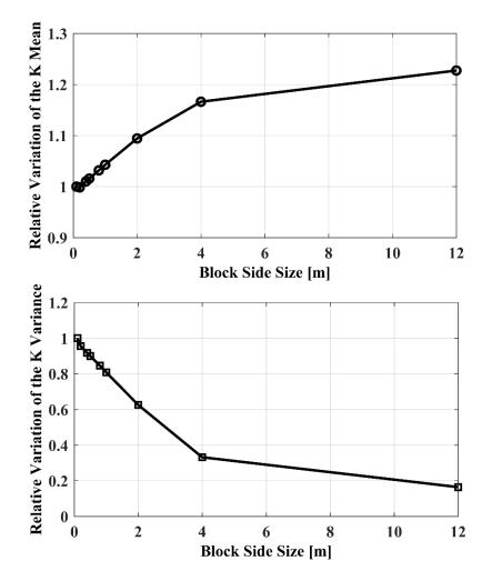
Fig. 4.6 Variation of the mean and the standard deviation of the upscaled conductivities relative to the mean and standard deviation of the fine-scale conductivity values
