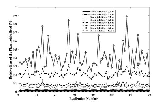
Fig. 4.7 Relative bias of head, RB<sub>h</sub>, for all block side sizes and all realizations when block values are computed with the Laplacian-with-skin upscaling method
