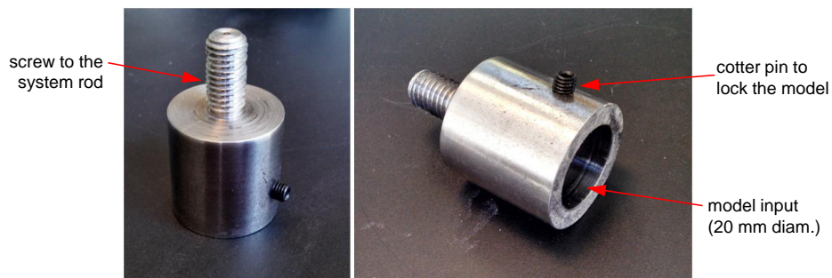
Figure 30. Coupling device.
