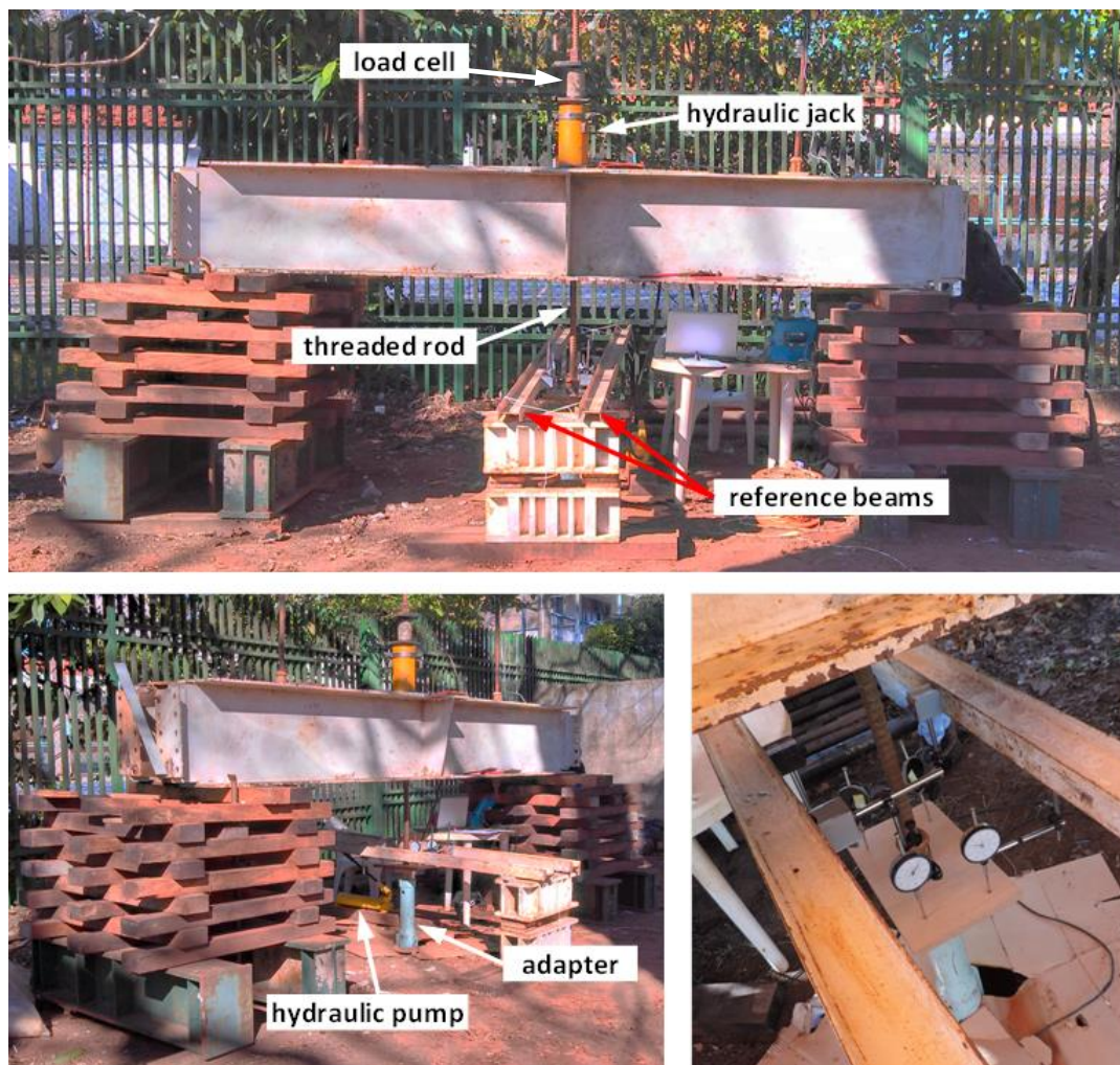
Figure 44. Load test setup.
