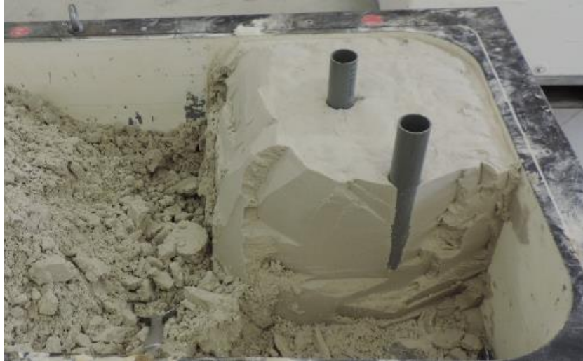
Figure 31. Extraction of specimens (with and without a model anchor).
