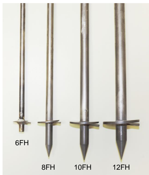
Figure 23. Helical model anchors with fixed helix.
