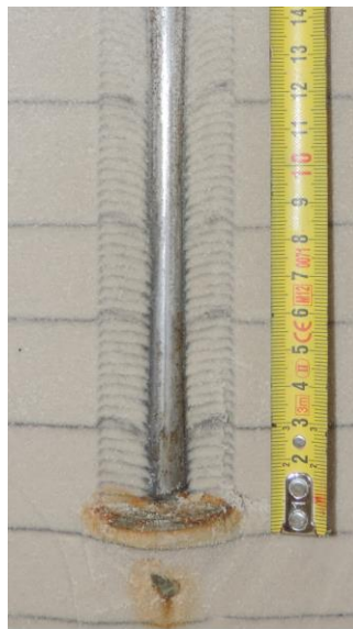
Figure 1. Photograph of a helical anchor model in very dense sand after installation.
