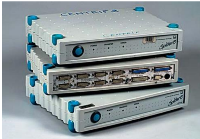
Figure 124. Spider data acquisition modules (Thorel et al., 2009).
