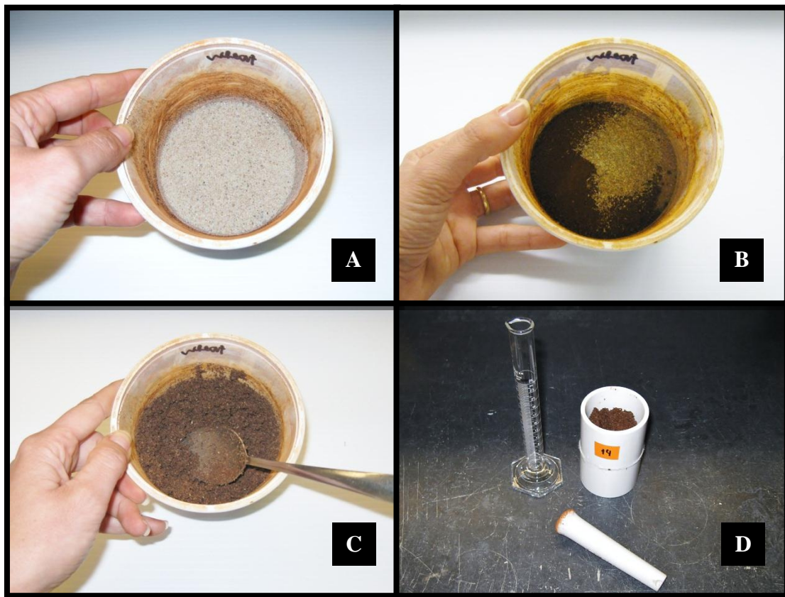
Figure 1 - Details of the open incubation experiment: Adding acid washed sand (A); Mixing with soil in equal weight and adding the plant residues (B); Bringing to 75% of the field capacity (C); Accommodating the material in PVC cylinders with a bulk density of 1.3 \text{ g cm}^{-3} (D)
