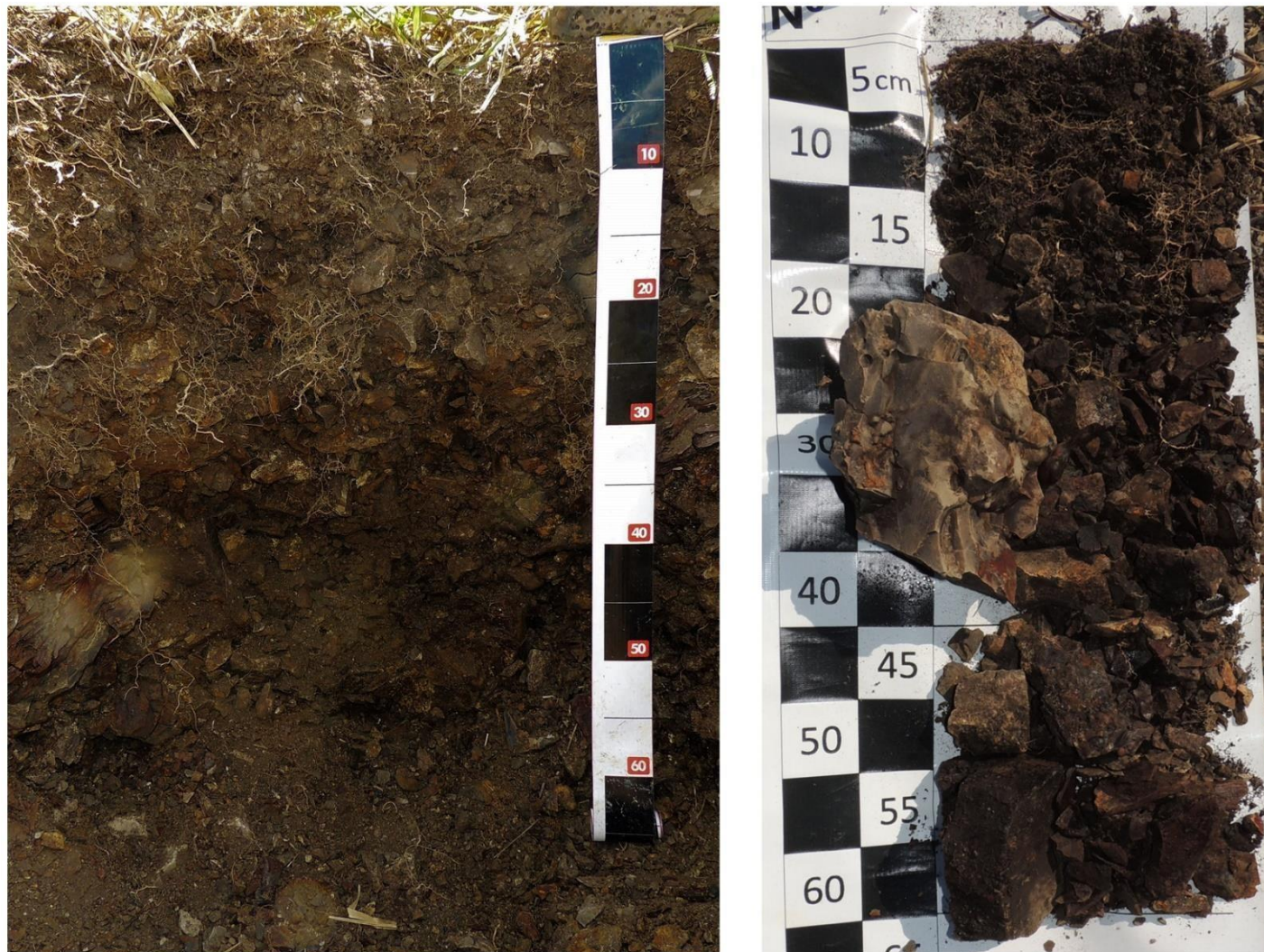
Fig A9) Soil profile from P20: Hyperskeletal Spolic Technosol (Hyperhumic, Loamic, Somerimollic).
