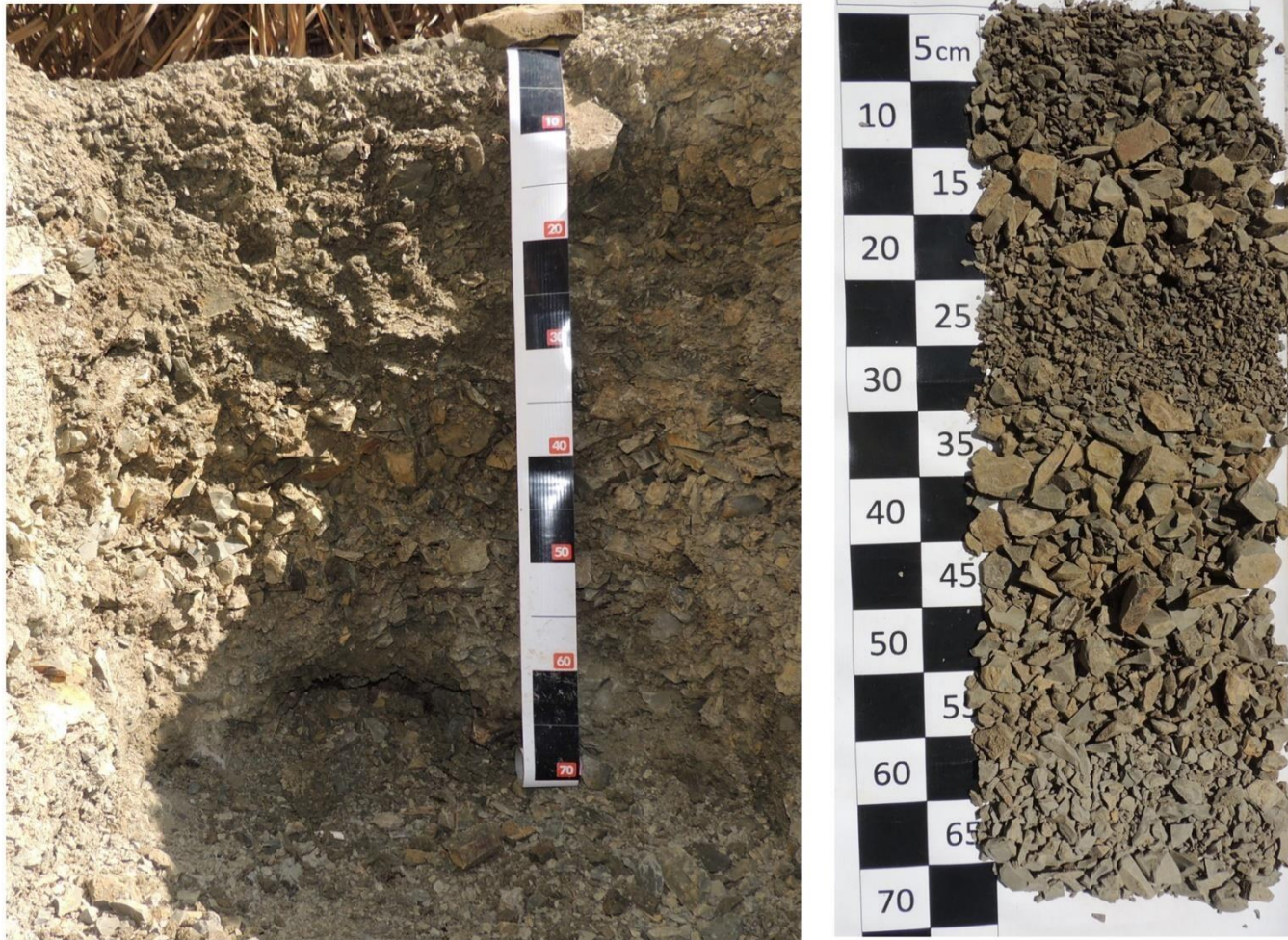
Fig A3) Soil profile from SC2: Hyperskeletal Spolic Technosol (Clayic)
